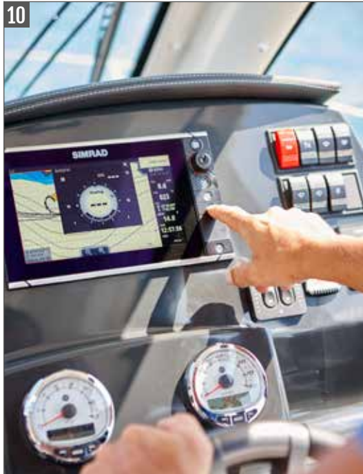
Integrated helm with SmartCraft instrumentation, mounting area for GPS/Chart Plotter
